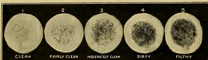
FIG. 2.—Filters from sediment tests showing the amount of dirt in different samples of milk. These are the grades made by the New York City Board of Health.
